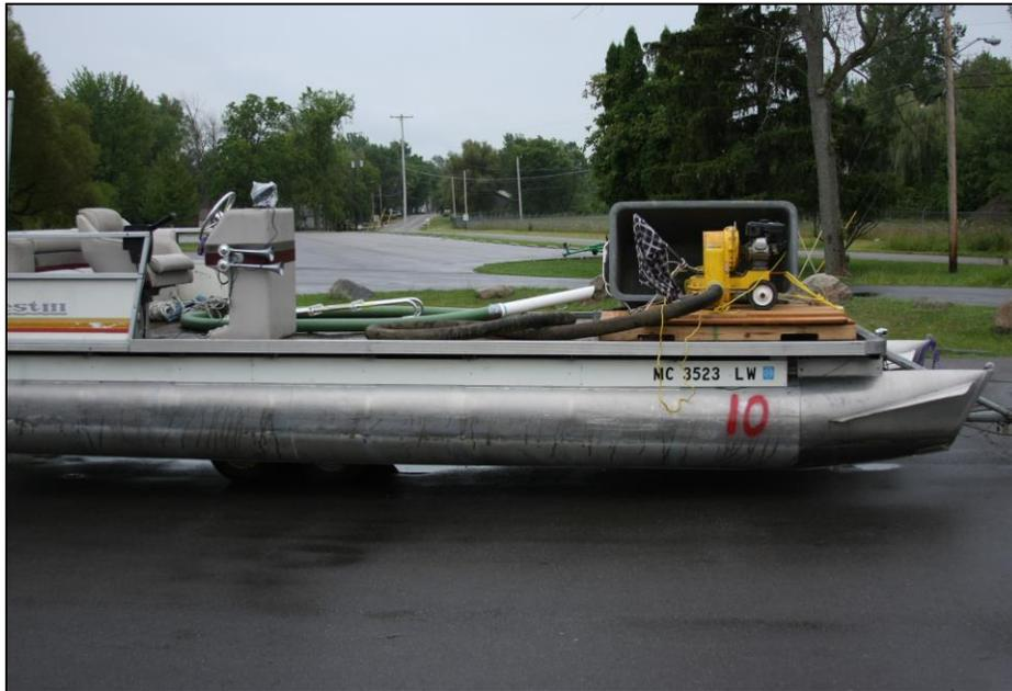
**Figure 57. A DASH boat used for aquatic plant removal (RLS, 2018).**
