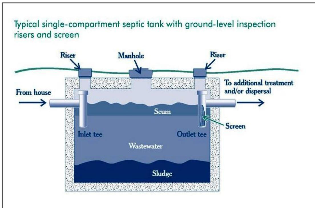
Figure 20. Diagram of essential septic tank components (US EPA).
