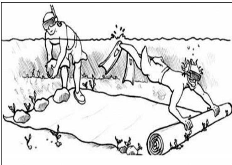
**Figure 55. A Benthic Barrier. Photo courtesy of Cornell Cooperative Extension.**
