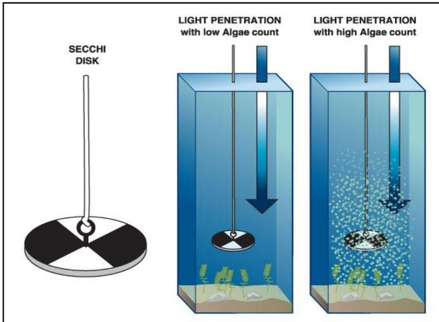
**Figure 12. Measurement of water transparency with a Secchi disk.**
