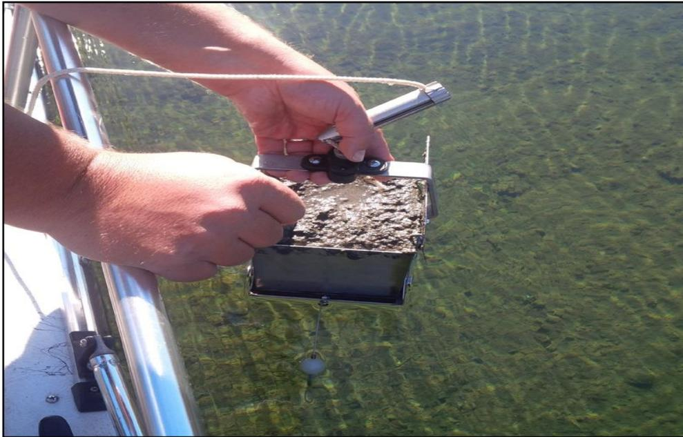
**Figure 45. An Ekman hand dredge for sampling lake sediments (RLS, 2018).**
