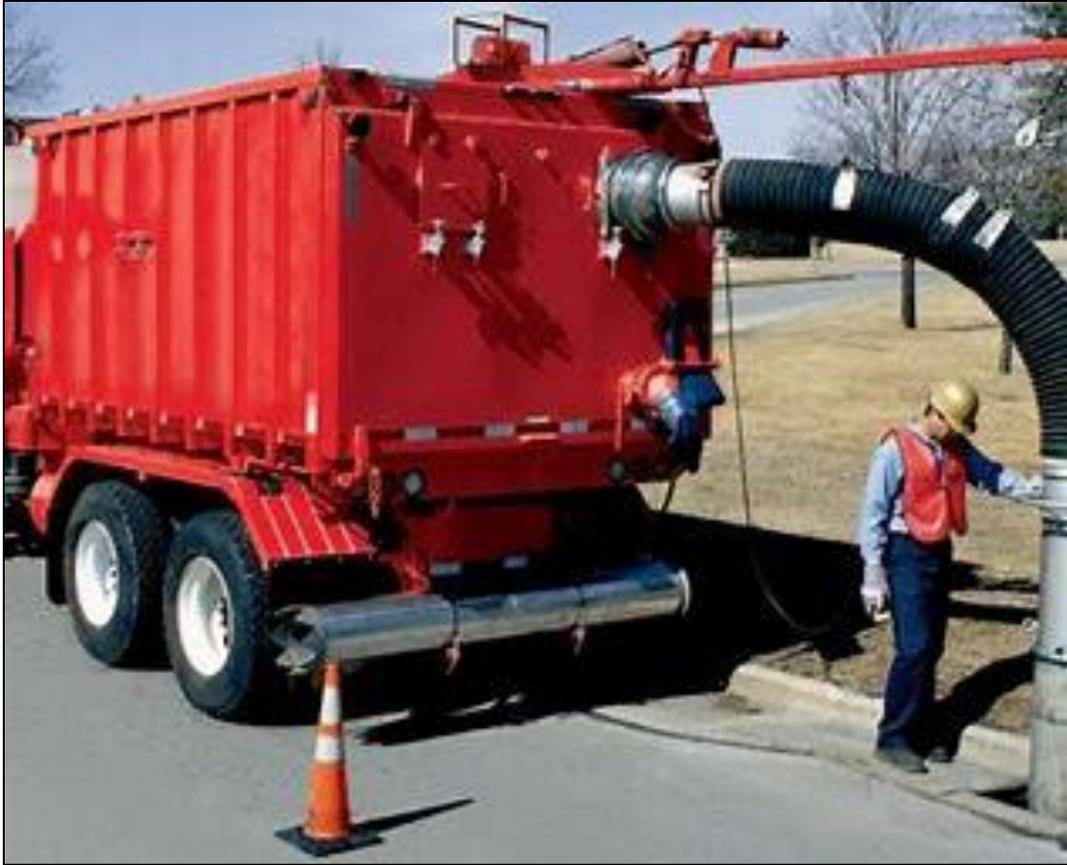
**Figure 32. Example of storm water maintenance (sewer cleaning).**
