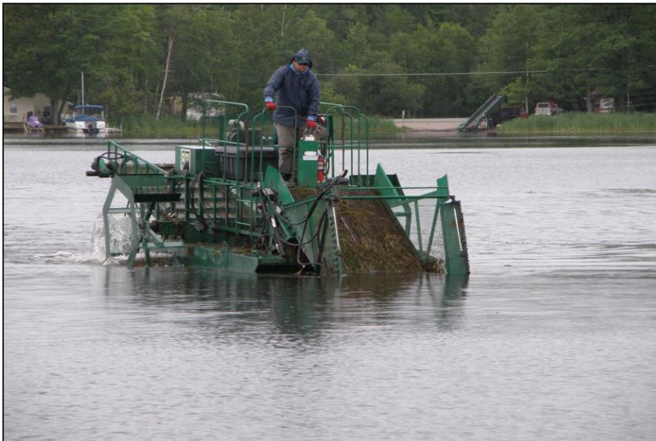
**Figure 54. A mechanical harvester used to remove aquatic plants (RLS, 2018).**
