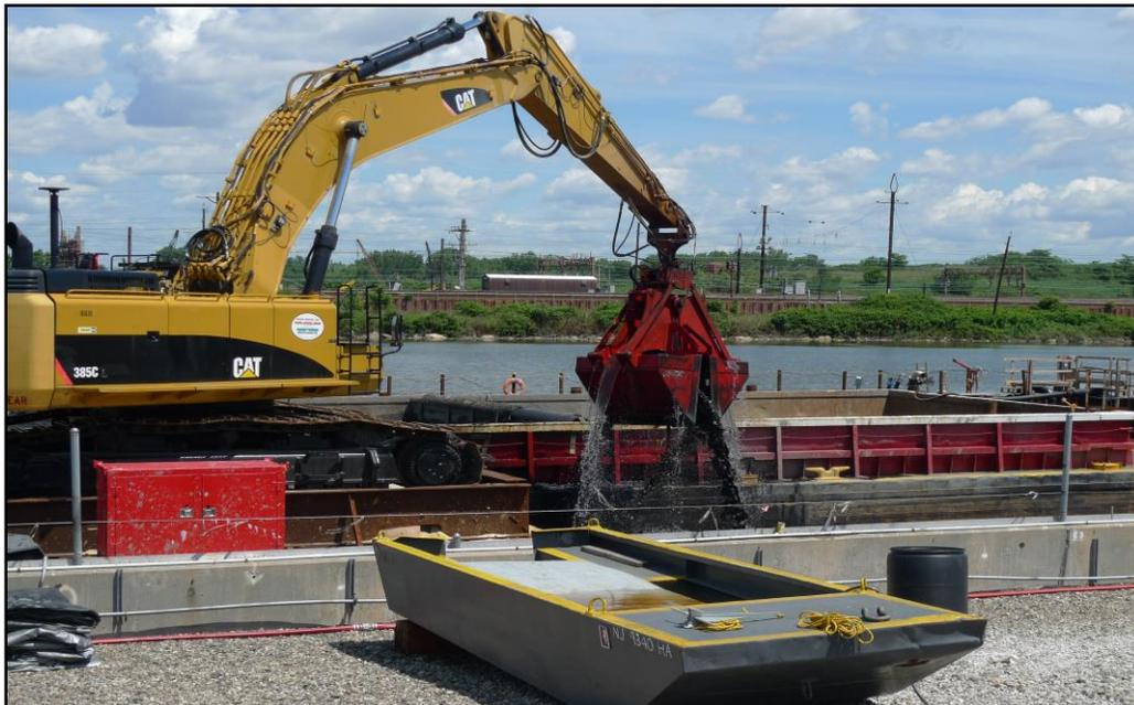
**Figure 59. A mechanical dredge for sediment removal in inland waters.**
