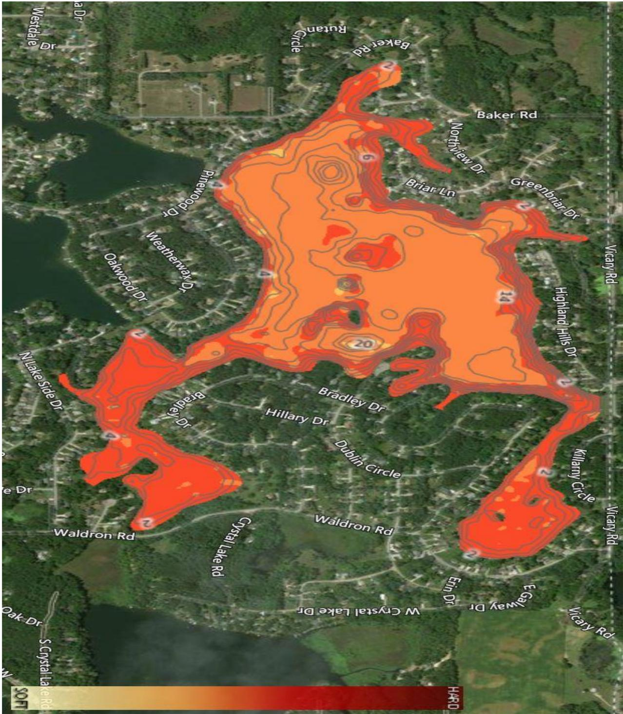
Figure 4. Lake LeAnn north basin sediment relative hardness map (September 11, 2019).
