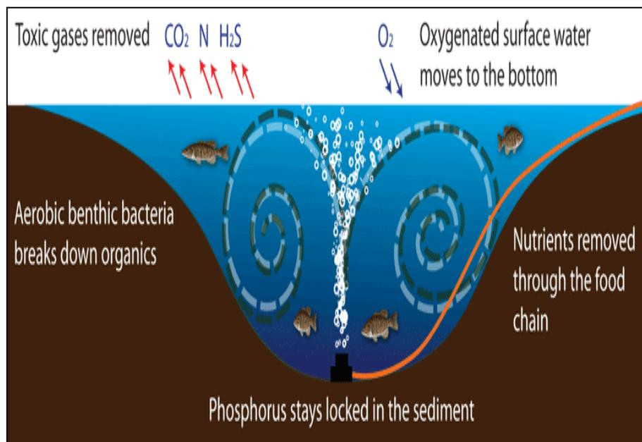
Figure 58. Diagram of laminar flow aeration. ©RLS
